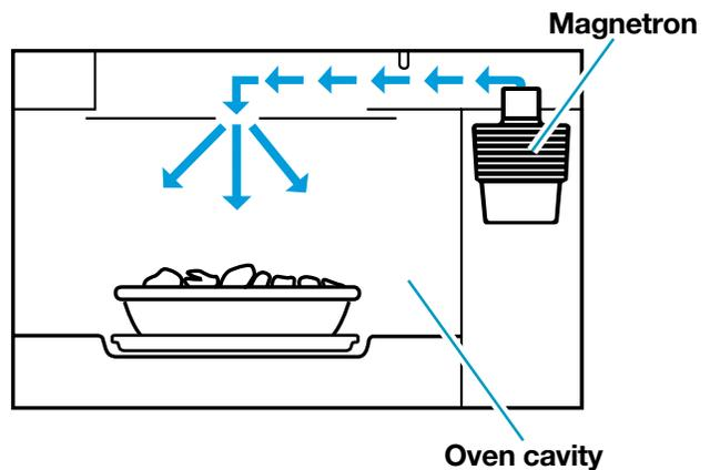
**The glass turntable** of your microwave oven lets microwaves pass through. Then they bounce off a metal floor, back through the glass turntable, and are absorbed by the food.
